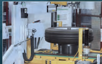
Retrofit of TU, geometry & balancing lines
