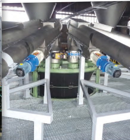
DOSING SYSTEM WITH FLEX SCALE HOPPER FOR BATCH INTEGRITY
